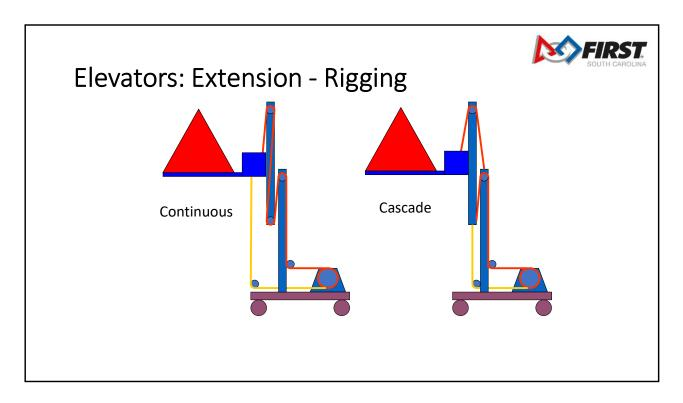
There are two primary ways to "rig" an elevator system.
