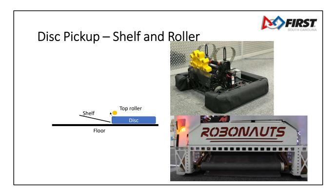
Flat objects definitely need an over/under approach for pick up. Typically this would be a piece of polycarbonate as a shelf / spatula and a powered roller on top to pull the piece toward the robot.
