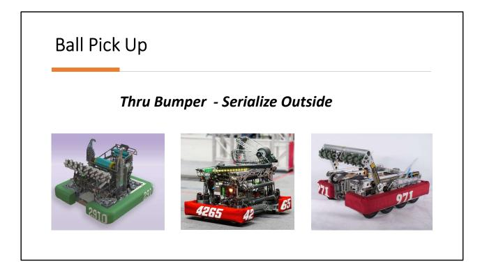
These robots "centered" the game piece while it was still on the floor before entering the robot internal conveyor system.
