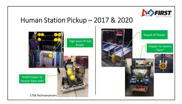
These are examples of human loaded machines. 1758's machine could also pick up balls from the floor through a bumper cutout. The foam balls were shoved up through the bottom hopper.
