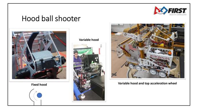
Shooting balls is also a common task in FRC. In all cases, I recommend using brushed DC motors like a NEO or Falcon with a closed-loop velocity control of the speed. This will be more accurate than only setting a specific percent output.
