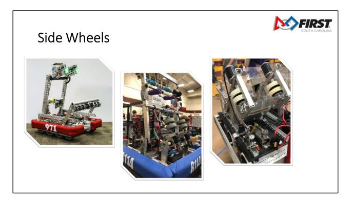
Side wheels can also be used to shoot a knuckle ball. Here, you need to be careful that both sides are running the same speed, or you could have inconsistent aim.
