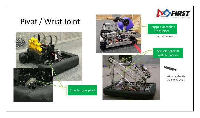
Pivots are usually chain powered as well. If the chain is short, it may be difficult to fit an inline tensioner. You can also do this with accurate center-to-center bearing spacing and not have to actively tension.
