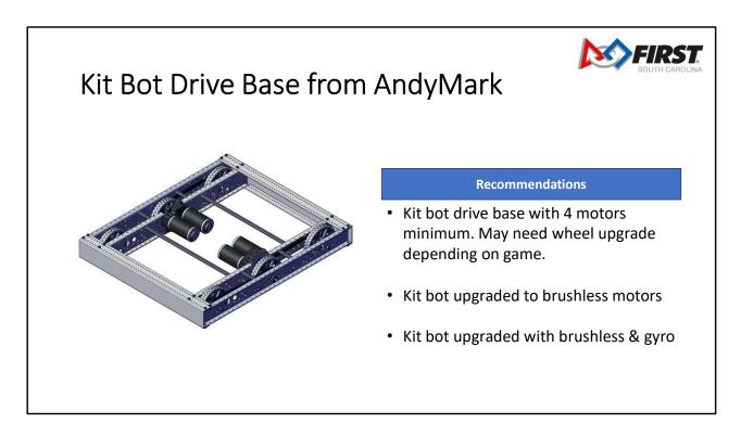
Kit bot drive is mechanically sound chassis for most teams. Recommend this is the first thing you build after review the FRAME PERIMETER rules and selecting the appropriate chassis size. The full size chassis will be too big. I recommend you leave the length the same and make it slightly narrower.
