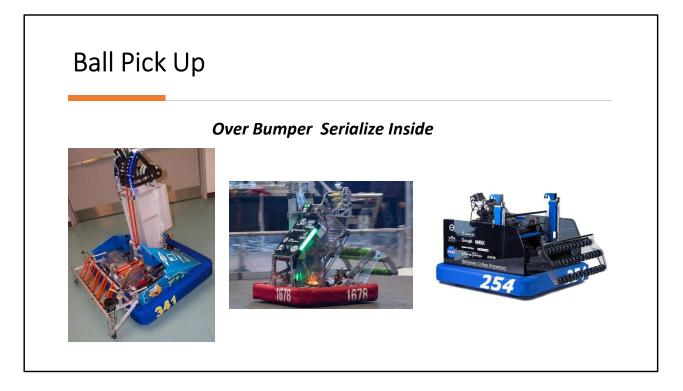
Another design approach is to bring balls in the robot over the bumper. PLUS: A wide intake zone makes it easy to pick up one or more balls without a lot of drive maneuvers. CON: One the ball is inside the bot, you need a hopper system to serialize the balls in a line before scoring.
