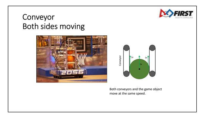
In both conveyor systems, please make sure the spacing between the belts is slimmer than the ball. It needs a little squeeze to hold it in the air. Usually an inch of compression should be fine.
