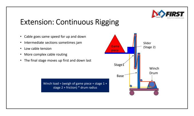
Method 1: Continuous rigging. There is one continuous cord (or belt) to go from the spool to the final stage. You can let gravity drop the elevator, but it is best to have a return pull down cable.
