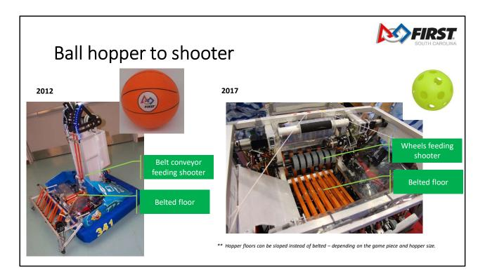
Serializing balls from a hopper into a linear conveyor to feed a shooter is a very common system in FRC. A completely gravity fed hopper usually is not effective. Using powered belts on the floor and/or sides of the hopper is needed.
