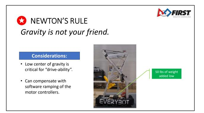
A well placed and low center of gravity (COG) make any drivetrain better performing and more controllable for the driver. High COG will show up as a tippy or unstable robot especially when starting or stopping. COG should also be near the center of the robot. If one end is heavy, it will be easy for the drive base to pop a wheelie.
