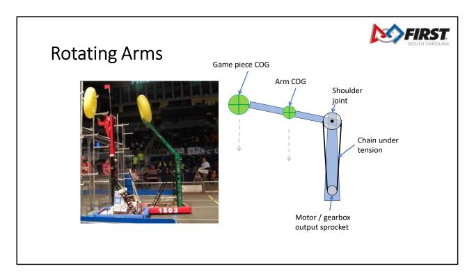
Rotating arms are also very common subcomponents of an overall system. This used as a big pivot (like above) or a small wrist joint or an intake pivot.
