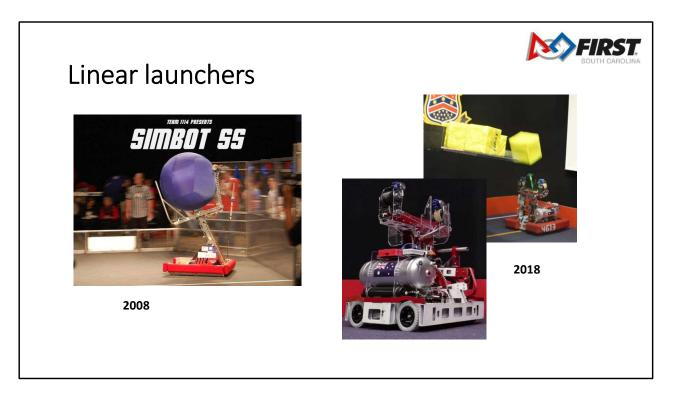
Another type of knuckle ball shooter is a linear puncher. This is usually powered by springs or rubber surgical tube. The 2018 example was a very unique solution that year since most teams used an elevator to score the game piece. Linear punchers were also used heavily in 2014 which had a similar yoga ball that 2008 used.
