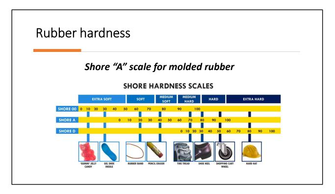
Most of the wheels used in FRC are rubber or rubber coated. The Shore A scale can be used to select good wheels for the game piece and task.
