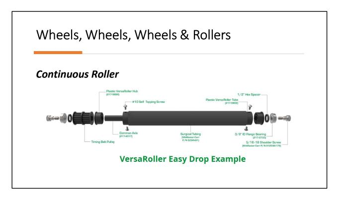
Full width rollers are also good for intakes and/or conveyors. Typically, these are hollow polycarbonate tubes. Team will cover the smooth rollers in grip tape or rubber to make them a bit more sticky.
