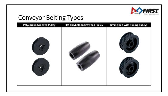
Polycord in grooved pulley: This is rounded poly cord you can buy from McMaster Carr or even some place like WestCoast products. NOTE: The round belt can jump out of the groove if there is side force on the cords. This system can be finicky.
