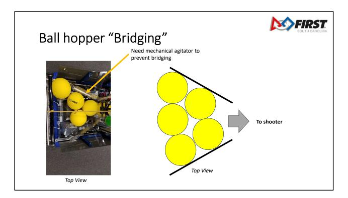
Gravity only may cause the balls to "bridge" where multiple balls can touch the hopper sides and get stuck without an active agitator. In the picture, a belt on one of the walls is used to prevent bridging.
